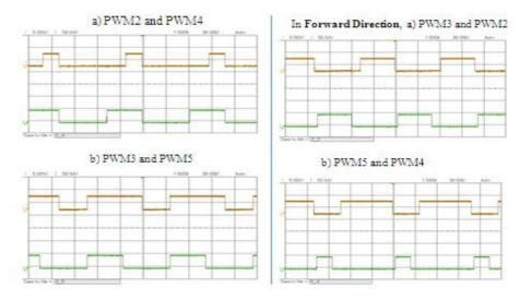
Fig. 6.4: Comparison of PWM2 and PWM3 with PWM4 and PWM5 at ADC=0
