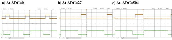
Fig. 6.1: PWM1 and PWM0 Waveforms
