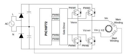
Fig. 2.1: PSC Drive with an H-Bridge
