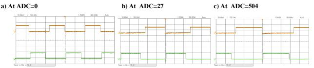
Fig. 6.2: PWM3 and PWM2 Waveforms
