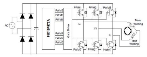
Fig. 3.1 Controlling a PSC motor with a 3-phase inverter bridge
