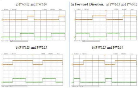
Fig. 6.5: Comparison of PWM2 and PWM3 with PWM4 and PWM5 at ADC=27
